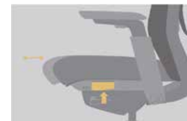
Adjust seat depth by 50mm
